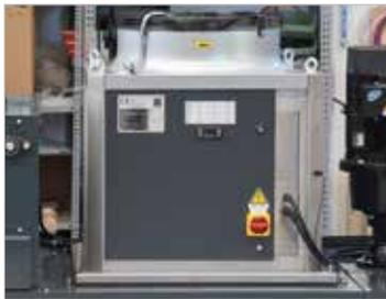
Submerged refrigeration unit to ensure the coolant temperature control;
