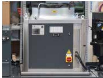
Submerged refrigeration unit to ensure the coolant temperature control;
