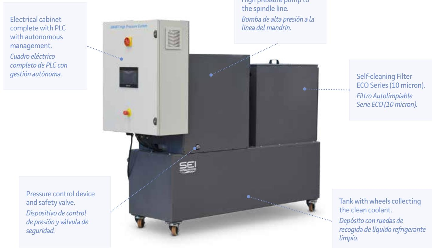
Recommended for lathes and work centers with internal induction of the minimum spindle 70 bar.
